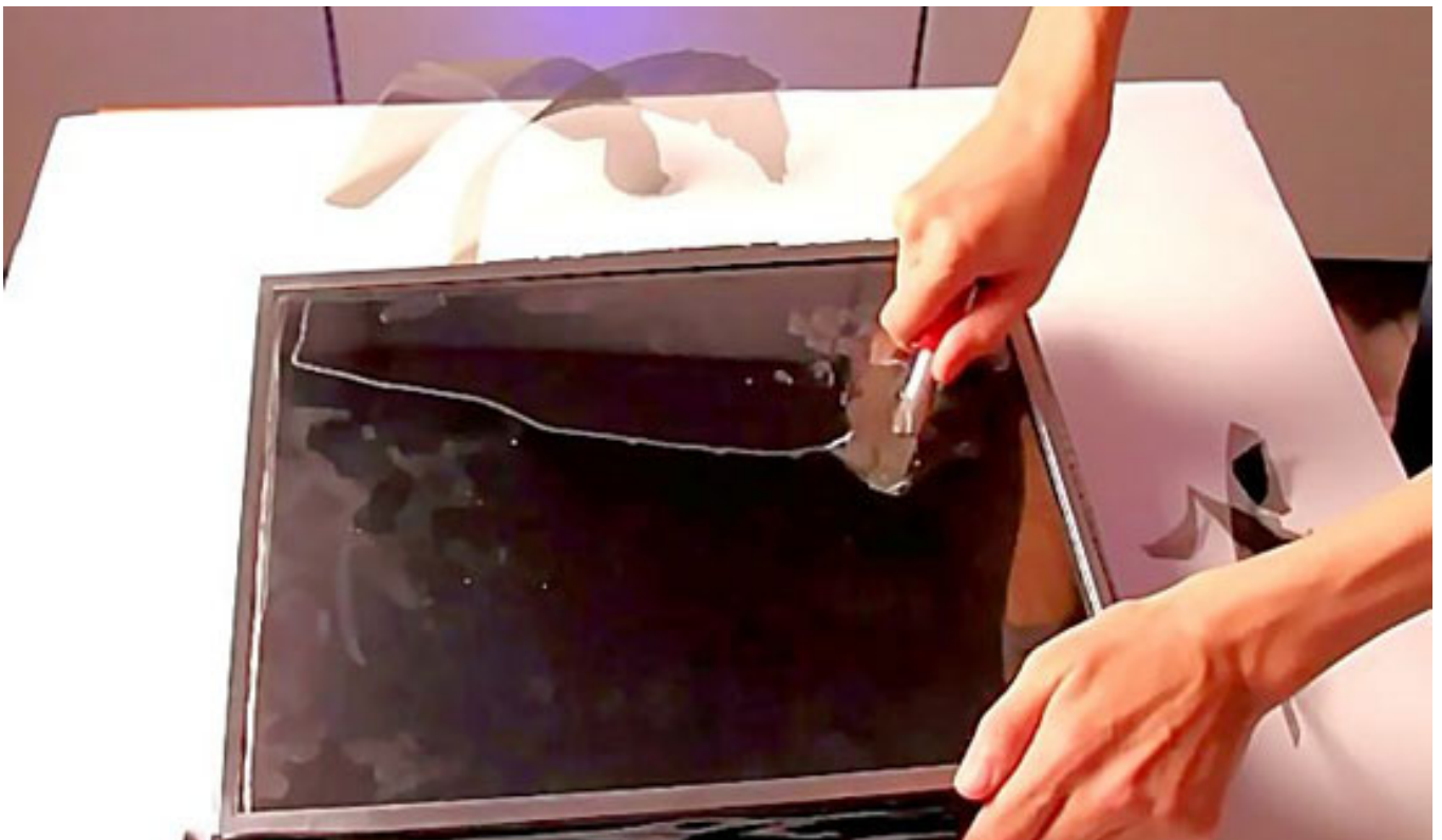
Brian Dodson demonstrates the process of removing the polarizing filter from an LCD display.
